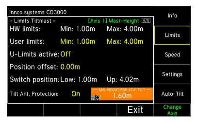
Figure 1.27: Limits Tiltmast
