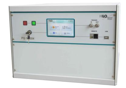
Compact EMC test unit designed for testing electromagnetic immunity of the electrical installation of vehicles and components against supply line transients.
