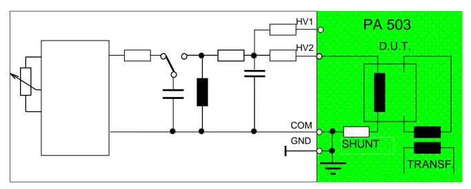
Fig. 2: Ring-Wave Generators IPG 612T, schematic, +Safety test cover PA 503, incl. modification of IPG 612T for testing RCCB's acc. to IEC 1008-1.
