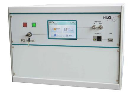
The oscillatory wave generator IPG 2554 has been designed for immunity testing of electrical and electronic equipment against repetitive damped oscillatory waves according to IEC 61000-4-18 requirements.
