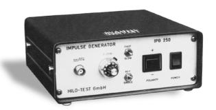
The pulse generator IPG 250 is designed for measuring the step response of high-impedance networks, for instance voltage dividers, oscilloscope probes etc. The generator excels by calibrated adjustment of output amplitude, short rise time and flat pulse top. The output pulse amplitude can be adjusted by use of a 10-turn potentiometer from 0 to 250 V. Positive and negative polarity can be selected.
