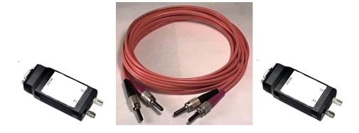
Fiber Optic Link Kit: FOLK- 01 – the low cost Option 2 solution to make fiber optic connection of Smart Fieldmeter to PC. Allows up to 100 ft. (30 meters) distance between screen room setup and equipment room PC. Kit includes two RS232/Optic converter units connected with bi-line fiber optic cable. Upstream converter unit is connected to PC Link Kit PCLK- 01- 1, while down-stream unit is plugged directly into RS232 port of the PC.
