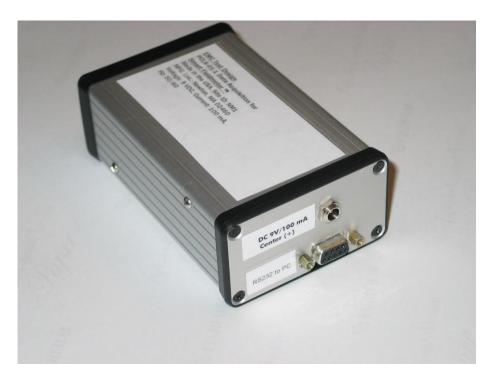
Introducing the Smart Fieldmeter PC Link Kit: PCLK- 01-1 – low cost Option 1 solution for simple connection of the Smart Fieldmeter to PC. This kit supports one Smart Fieldmeter unit and has into one stylish metal box containing the isolating differential amplifier (with more than 120 dB AC decoupling) and DAQ module acquiring 120 samples/sec with RS232 PC output. Software for data streaming, recording and archiving is included.
