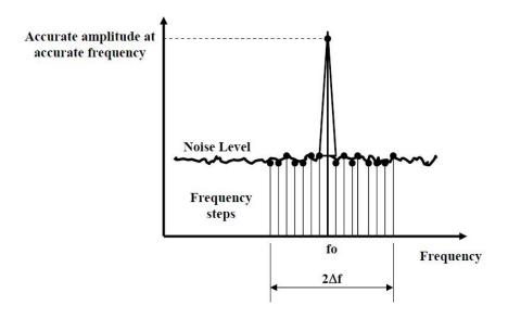
Figure 4. The DSI technique for cheap frequency "tracking" measurements
