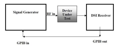
Figure 3. Swept frequency tracking with a DSI Receiver
