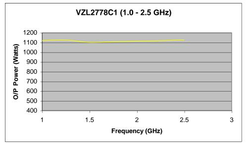
Figure 4(a): VZL2778C1 (1.0-2.5GHz, 1000-Watts) O/P Power versus Frequency
