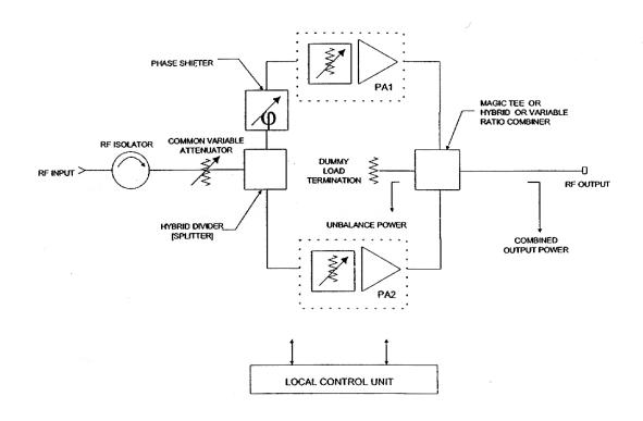
Figure 1. Block Diagram, Basic Power Combiner Circuit
