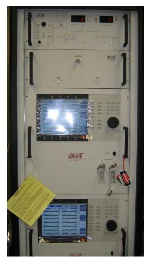
Along with the TWTA RF source specified herein, the series of power/phase combiners consist of a coaxial input divider network, phase shifter, and a front panel module. The front panel combiner module comes equipped with the following features:
