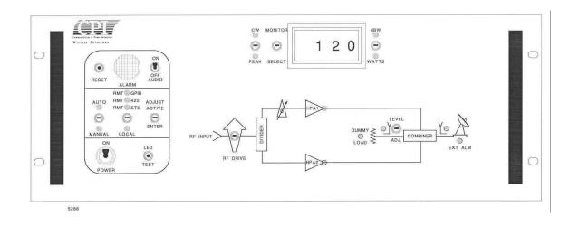
Figure 3: Power Combiner Module Front Panel
